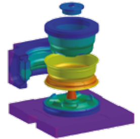
Low Pressure Die Casting of an Alloy Wheel
