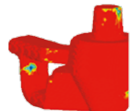
Unfilled or poorly compacted areas
