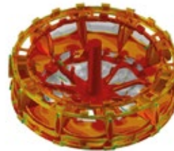
An engine casing cast using centrifugal process
