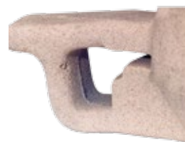
Unfilled or poorly compacted areas
