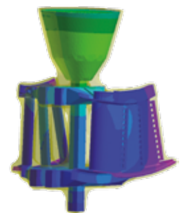
NGV Blade with Realistic Shell Modelling
