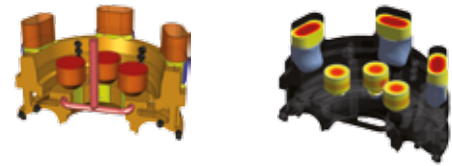
Final design after 5 iterations showing no more hot spot in the part.
